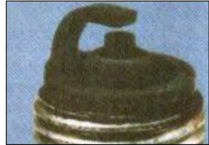
Fig. 89-Spark plug fouled with soot
