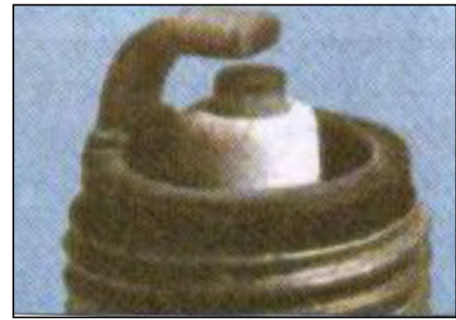
Fig. 88-Spark plug in normal condition
