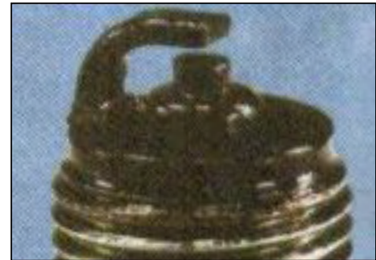
Fig. 90-Spark plug fouled with oil
