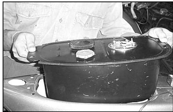
Fig. 185-Lifting out the tank from frame
