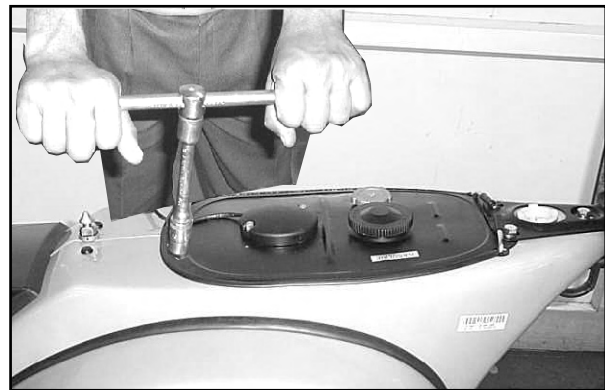
Fig. 184-Loosening securing bolts of petrol tank
