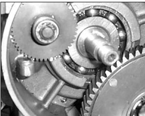
C.- Place plain washer and lock with circlip
