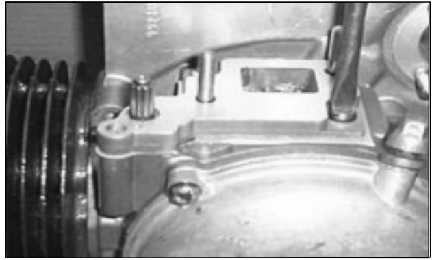
Fig. 177-Mounting the air cleaner case
