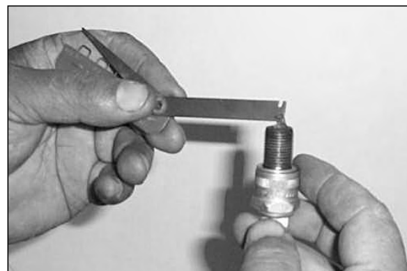
Fig. 87-Resetting the spark plug gap
