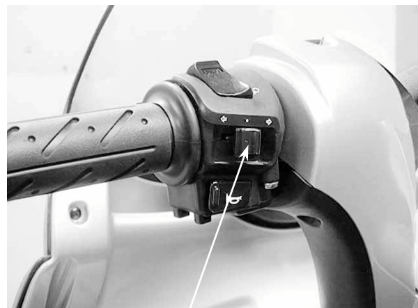
Turn Signal Switch
